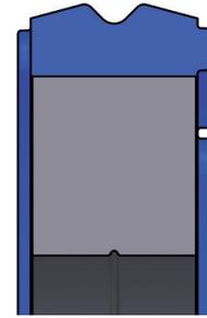
The double-acting K84 is composed of a highly extrusion-resistant TPU sealing element, which is prestressed by a rectangular NBR ring. The K84 is distinguished by its extraordinary sealing function under both dynamic and static loads. If there is pressure on both sides, two sealing edges establish a secure media separation.
